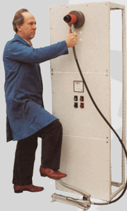
Pressure release is by means of a toe operated side lever to avoid bending down.
