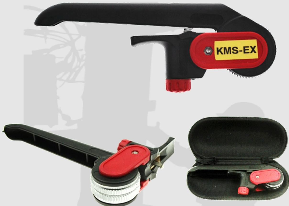
Designed for the removal of the outer XLPE sheath quickly and easily on all large size cables with a ratchet up and down action the stripper moves along the cable cutting the sheath as it goes.
