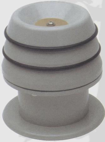
This Tool is used for visual inspection and to inflate the gloves to test for any air leaks.
