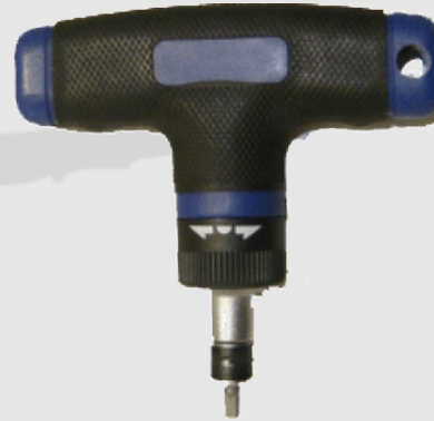
4mm Tamper In-Hex Insert Bit for the old Street Lights
